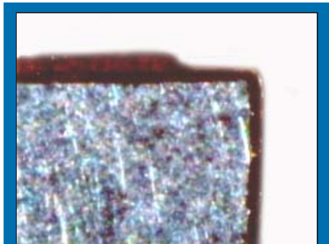
Magnified sectioned view of Anotherm™ substrate and trace. The anodized insulation layer gives excellent continuous coverage, even around sharp corners
